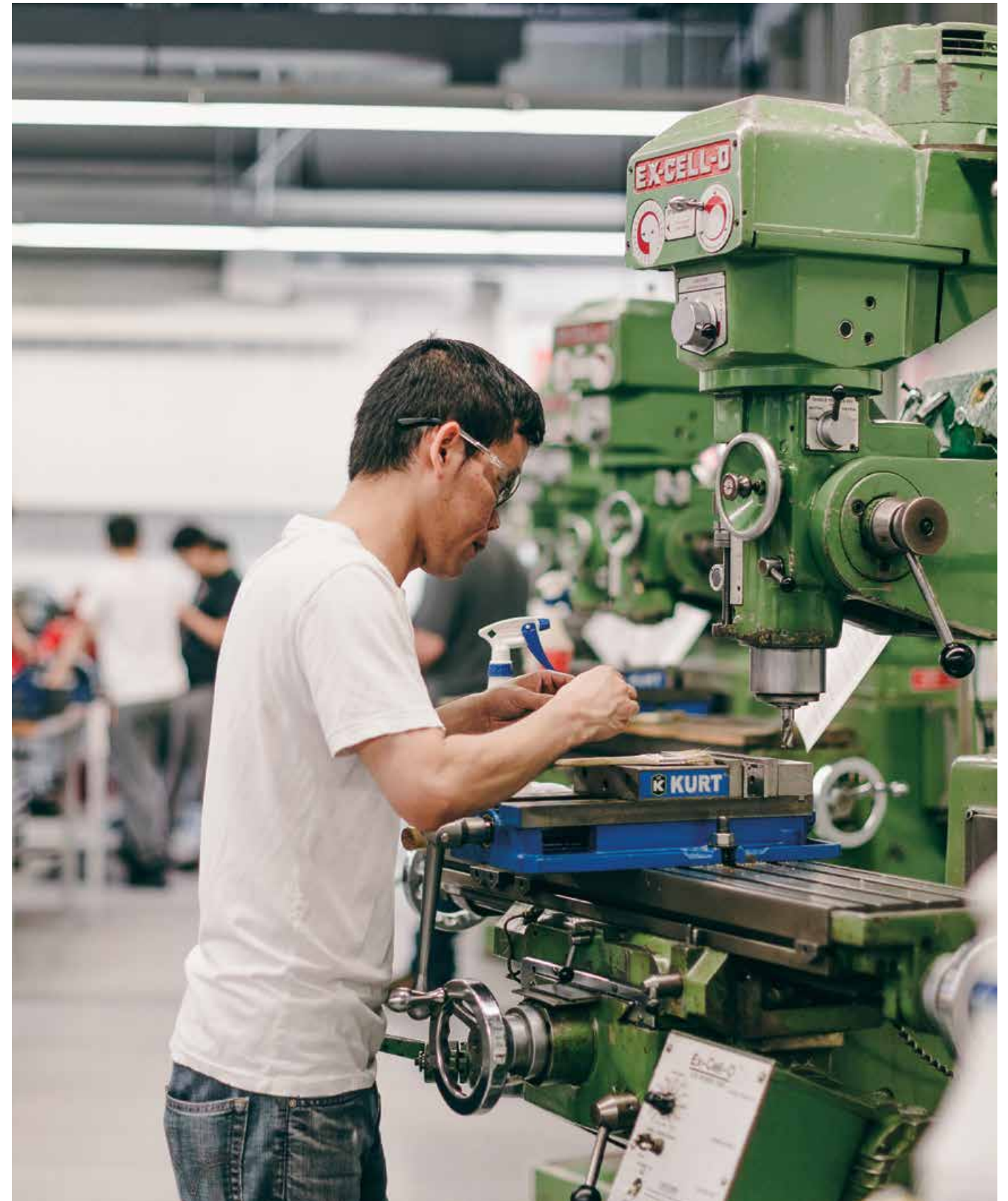
PICTURED ABOVE: A student learns how to use a conventional milling machine to complete machining operations.
